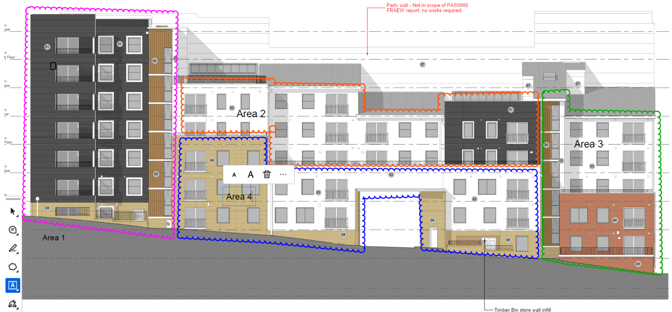
Piran – Sequential areas for façade removal
